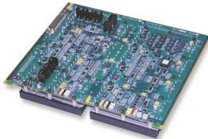
F-2015: Multiple Output Power System for Ground-based Test Equipment
